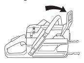
**Starting:** The chain brake must be engaged when the chain saw is started. Activate the brake by moving the front hand guard forwards.
